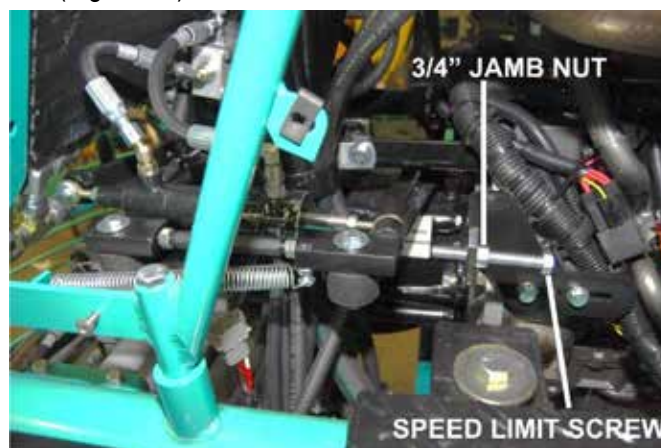
Figure 32. Left Side Trowel Speed Adjustment
